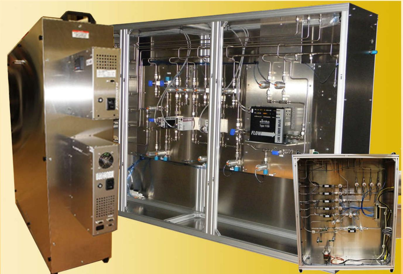
**FLOCON series gas and vapour flow management systems are highly versatile and economical tools for advanced CVD, PVD and PECVD process development, as well as variety of other applications. A sophisticated computercontrol system allows programming the flow rates, ON/OFF timing and duration of individual flow controllers, using a user friendly graphic interface. Option to integrate FLOCON into a Process Management system is feasible.**
